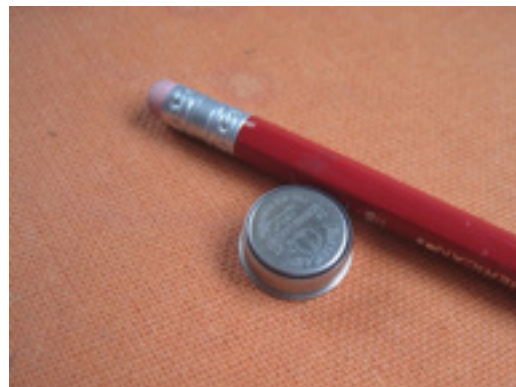
An i-Button body temperature logger. These are surgically implanted under the skin.
