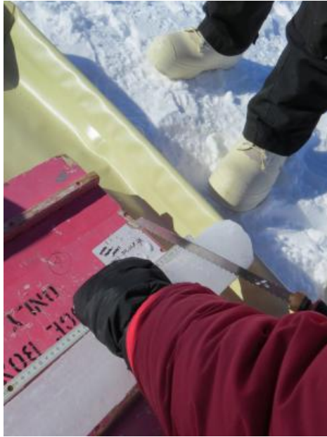
Sawing ice cores in the field
