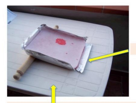
freeze water mixed with colored gravel in a basin (the gravel simulates the sediments transported by the glacier)
