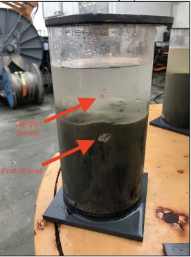
A HAPs core with an oxygen sensor that will relay data on the oxygen consumption of organisms in the mud core.
